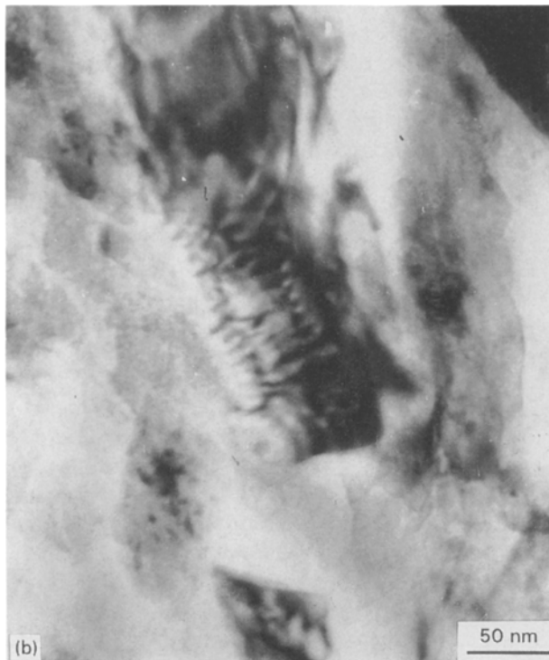
Figure 8 SEM micrograph of the release wave zone layer of particles (200–315 μm).
