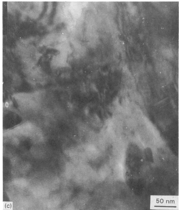
Figure 7 TEM analysis of shock compacted AlMgSi 0.5 . (a) the interparticle contact area; (b) the matrix structure of spheres; (c) the substructure of the interparticle contact area.
