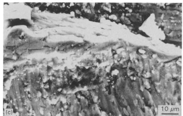
Figure 6 SEM micrographs of the zone of planar impact in the last layer of particles 200–315 \mu\text{m} (a) and (b) the impact zone; (c) magnified detail of the melted area.
